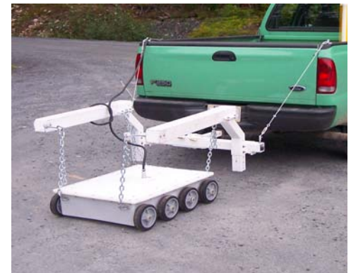
VIS-1 Vehicle Installation System (Shown with Model 301B Antenna)
