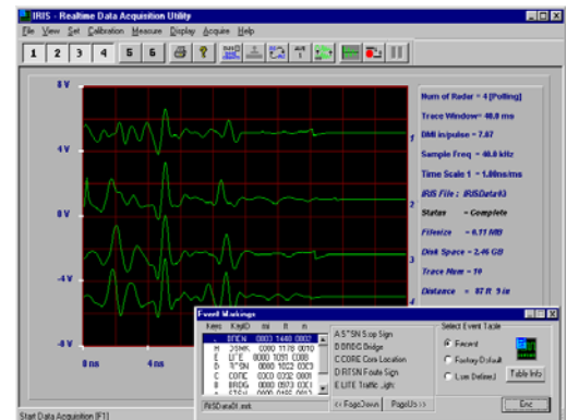
Data Acquisition Software (RDA) (for real-time data collection/display/storage)
