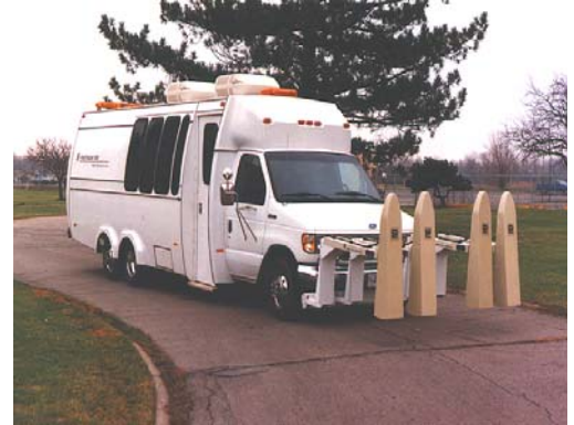
IRIS Minibus Vehicle (shown with 4 antennas)
